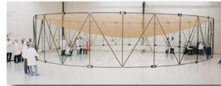
TRW AstroMesh antenna
