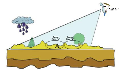
Dynamic, real time, in-situ measurements allow validation of satellite generated estimates of average soil moisture
