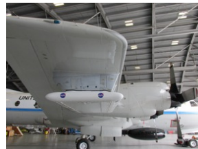
EcoSAR antenna (1 out of 2 shown) integrated to NOAA P3 aircraft
