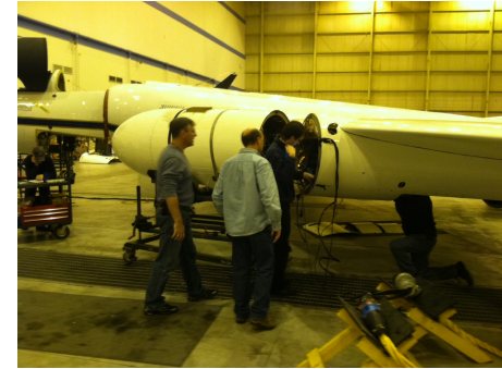
CATS instrument installation in ER-2 superpod Left: integrated in the forward superpod Right: final check and fit before flight
