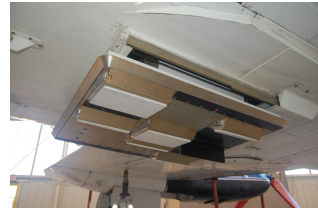
AirSWOT antenna subsystem mounted on King Air B200 aircraft.
