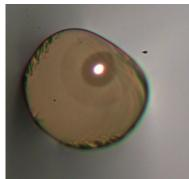
Example of broadening of the Brillouin gain through the development of an off-center core  $P_2O_5$  fiber with a special carbon fiber jacket that allows it to be spooled tightly resulting in a passively varying stressed fiber
