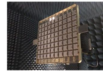
DBSAR's L-band phased-array antenna will enable meter-resolution and fully polarimetric measurements of permafrost and biomass
