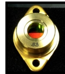
Packaged CW DFB laser with TEC
