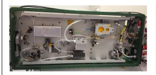
Thulium Fiber laser pumped Holmium-only two micron laser in a ring cavity configuration with demonstrated operation at pulse repetition rates from 100-1 kHz at output powers from 4-8 Watts
