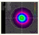
Injection seeded, single frequency beam profile
