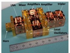
The dual-polarized, sideband separated receivers at 180-270 GHz (left) and 620-660 GHz (right) developed using HEMT-based amplifiers and multipliers. They require 20K cooling, as compared to superconductor-insulator-superconductor (SIS) receivers which need to be cooled to 4K.
