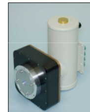
Mounted in Liquid N 2 Dewar for Operation at 77 K
