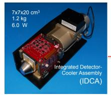
2x8 pixel linear mode photon counting HgCdTe avalanche photodiode detector with microlens array in a mini-Stirling (tactical) cooler
