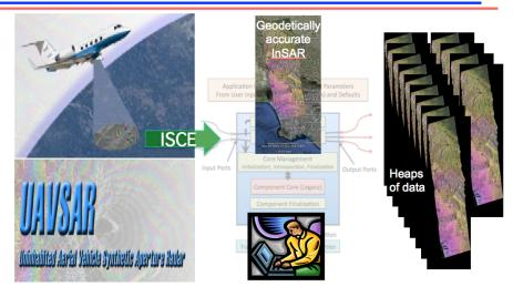
Production of geocoded deformation fields from UAVSAR interferograms and stacks of single look complex images via ISCE
