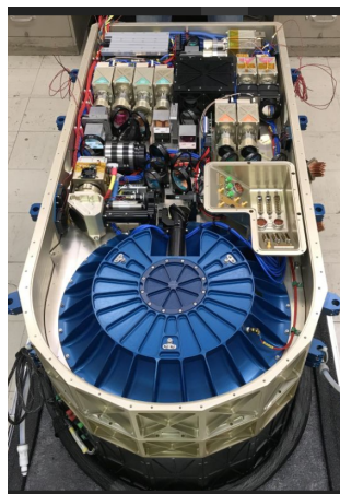
Above: HSRL lidar with ocean and aerosol channels. Above right: flight interferometer. Bottom right: detector package for the high-speed ocean surface return.
