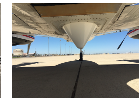
DopplerScatt prototype mounted on King Air B200
