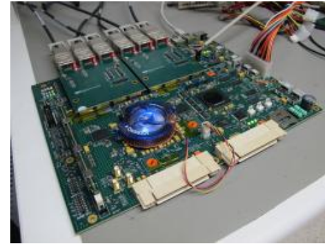
ROACH-II board with integrated Xilinx Virtex-6 FPGA available for high speed digital processing
