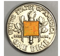
SiGe GNSS receiver chip layout (top) and fabricated chip (bottom)
