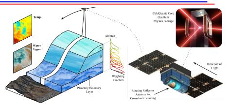
A QuARREM-based microwave radiometer flight concept with a ColdQuanta quantum sensing platform as the core "backend microwave electronics". The concept would operate in a cross-track scanning mode using a rotating reflector antenna to satisfy spatial sampling requirements for free atmosphere, PBL, and surface imaging science.
